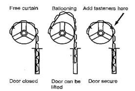
2. Lead in on tracks must **not** be folded back down hard on track. This defeats the purpose of them, which is to guide the door curtain in a smooth motion.
